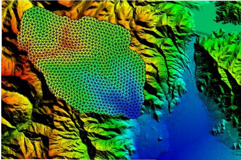
Figure 16 Interpolated TIN based on raster catalog
