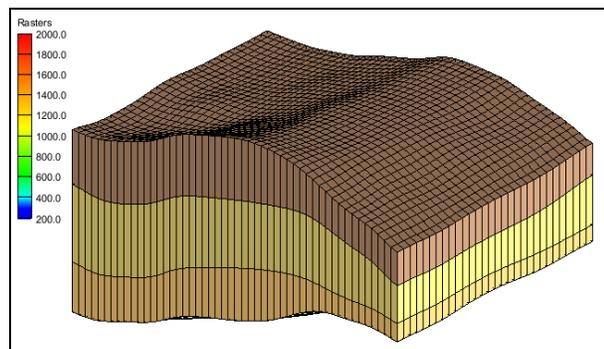
Figure 19 MODFLOW layers after interpolating elevation data
